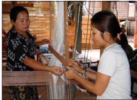
Figure 17. Eui Kim (left) and Dalounny Phonsouny (right) connecting the ends of a placeholder string to the nails on the posts
