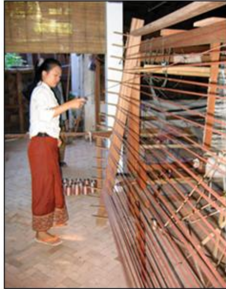
Figure 8. Sun winding the first meters of silk onto a warping frame
