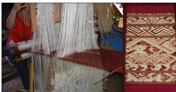
Figure 30. The use of two long heddle systems for storing an elephant’s design
