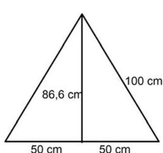
$$\begin{aligned} C^2 &= h^2 - C^2 \\ C^2 &= 100^2 - 50^2 \\ C^2 &= 10000 - 2500 \\ C &= \sqrt{7500} = 86,6 \end{aligned}$$
